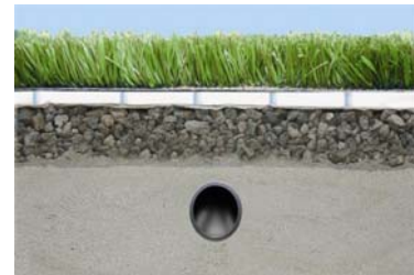
The Alveo Sports Layer (shown in white in the graphic) forms the flexible technical base layer for the layer system between the subbase and artificial grass fibre.
